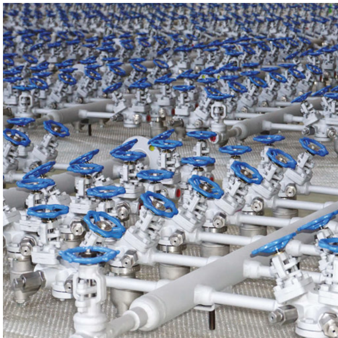
A "sea" of manifolds including valves and steam traps manufactured in Velan India and shipped to a chemical plant in Canada.
