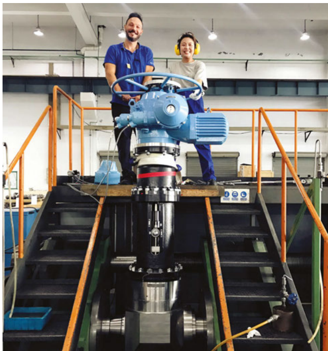
That's teamwork! Manufactured by Velan S.A.S. in France, this valve was sent to Velan China's Suzhou plant for hydrotesting before reaching its destination in one of China's nuclear power plants.
